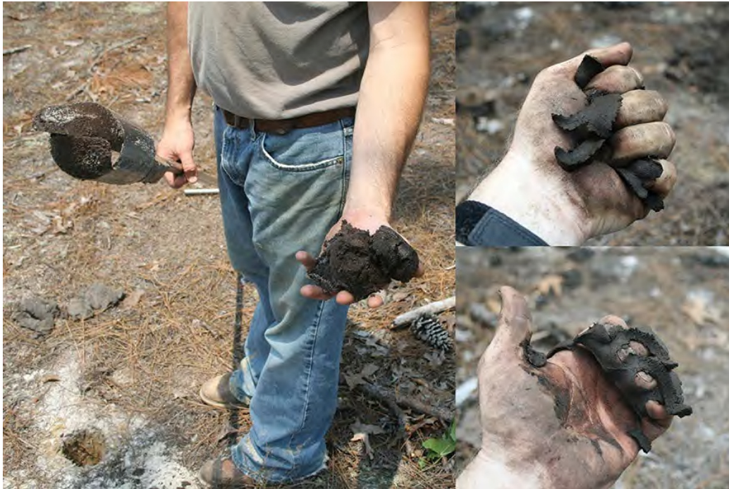
A field test on a soil with a moderately fluid manner of failure class. (Photo courtesy of John Kelley)
